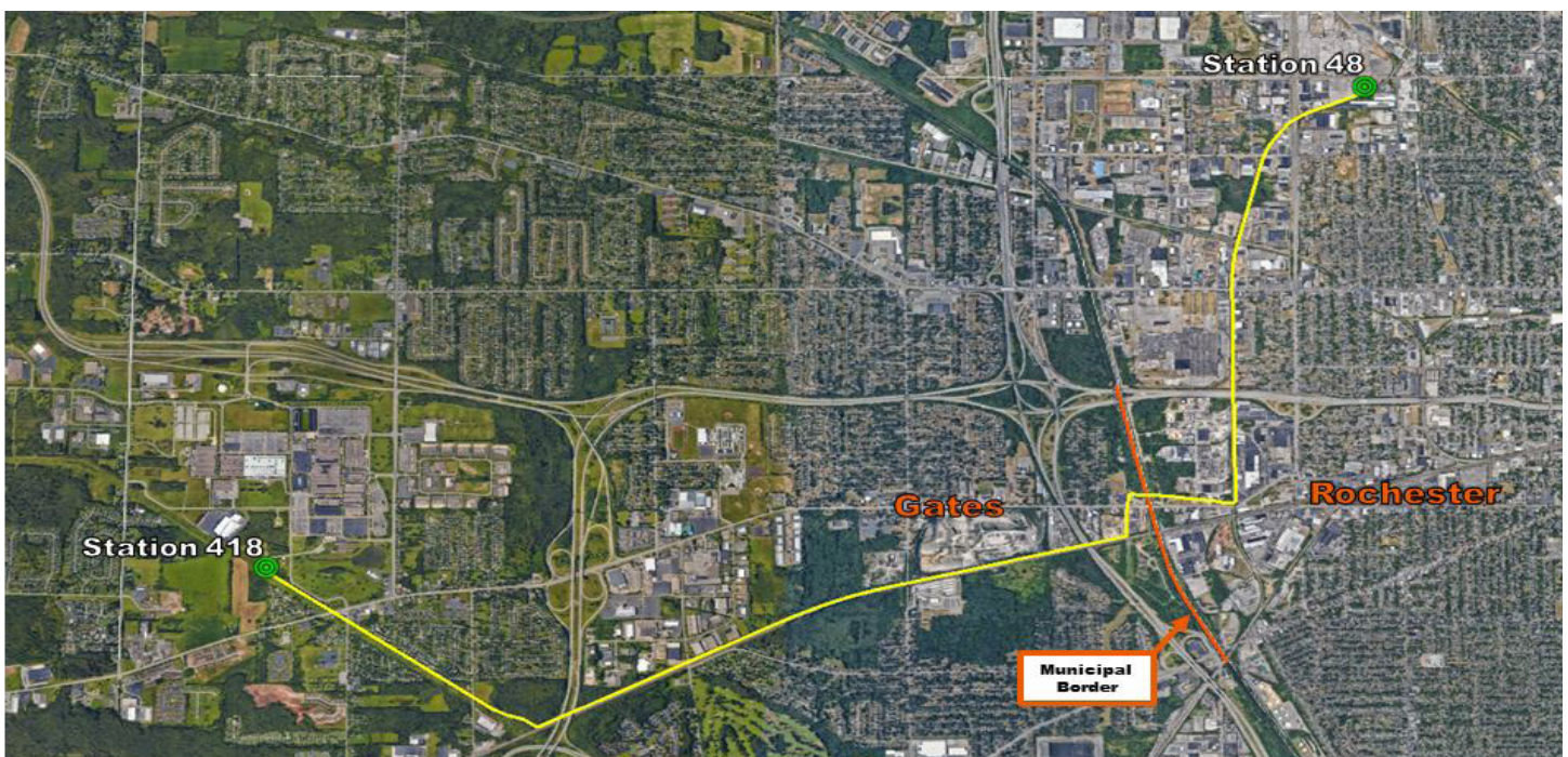
Planned route of new transmission line (L949) between Station 418 in the Town of Gates and Station 48 in the City of Rochester.
